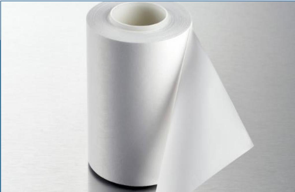
An e-PTFE Membrane is created when PTFE — a linear polymer consisting of fluorine and carbon molecules — is expanded, creating a microporous structure with very desirable characteristics, including a high strength-to-weight ratio, biocompatibility, high thermal resistance, and many others: Attributes. High porosity.
