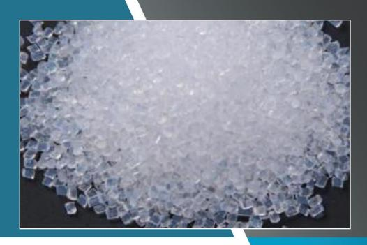
Fluorinated ethylene propylene (FEP) is a copolymer of hexafluoropropylene and tetrafluoroethylene. It is a transparent polymer that remains elastic at low temperatures. FEP is highly resistant to chemicals, as well as to aging and climatic influences. This polymer also boasts good dielectric properties with a minimal dielectric constant.
